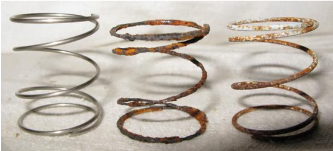
The spring on the left is in good condition. The other two need to be replaced.
